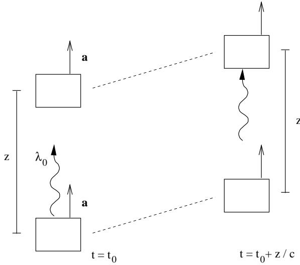
The boxes remain a constant distance apart, so the photon reaches the leading box after a time  $\Delta t = z/c$  in the reference frame of the boxes. In this time the boxes will have picked up an additional velocity  $\Delta v = a\Delta t = az/c$ . Therefore, the photon reaching the lead box will be redshifted by the conventional Doppler effect by an amount
