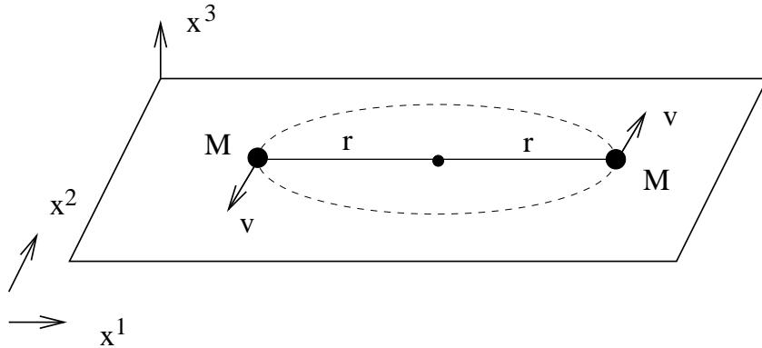
We will treat the motion of the stars in the Newtonian approximation, where we can discuss their orbit just as Kepler would have. Circular orbits are most easily characterized by equating the force due to gravity to the outward “centrifugal” force:
