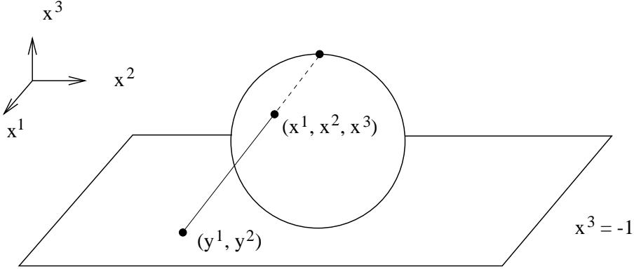
Thus, we draw a straight line from the north pole to the plane defined by  $x^3 = -1$ , and assign to the point on  $S^2$  intersected by the line the Cartesian coordinates  $(y^1, y^2)$  of the appropriate point on the plane. Explicitly, the map is given by
