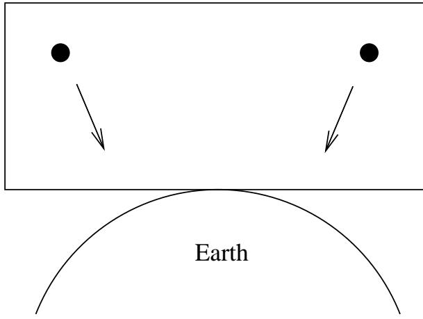
The WEP can therefore be stated as “the laws of freely-falling particles are the same in a gravitational field and a uniformly accelerated frame, in small enough regions of spacetime.” In larger regions of spacetime there will be inhomogeneities in the gravitational field, which will lead to tidal forces which can be detected.
