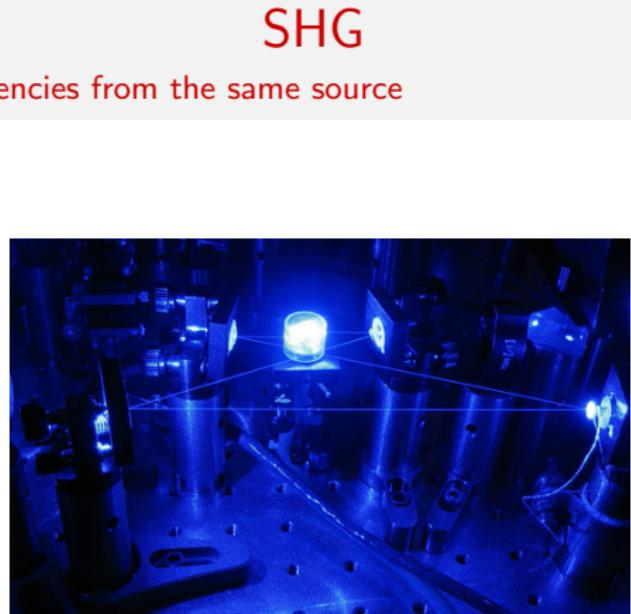
Figure: Closeup of a BBO crystal inside a resonant build-up ring cavity for frequency doubling 461 nm blue light into the ultraviolet. ([source flickr](#))
