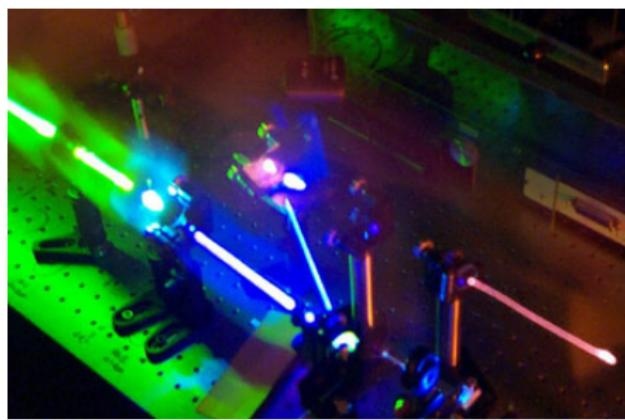
**Figure:** White light continuum seeded optical parametric amplifier (OPA) able to generate extremely short pulses.
