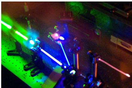
Figure: White light continuum seeded optical parametric amplifier (OPA) able to generate extremely short pulses. (source Freie Universität Berlin)
