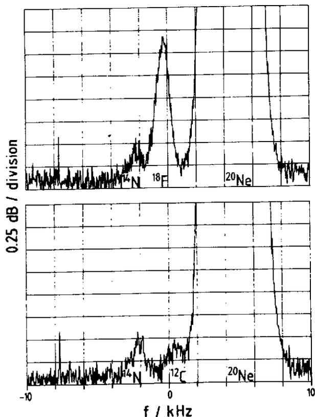
FIG. 33 Schottky spectrum at the 49th harmonic of the revolution frequency of 250 MeV/nucleon  $^{18}\text{F}$  fragments measured directly after injection and cooling (top) and 12 h later (bottom). The maximum of the  $^{18}\text{F}$  frequency distribution was at 83 293 kHz.
