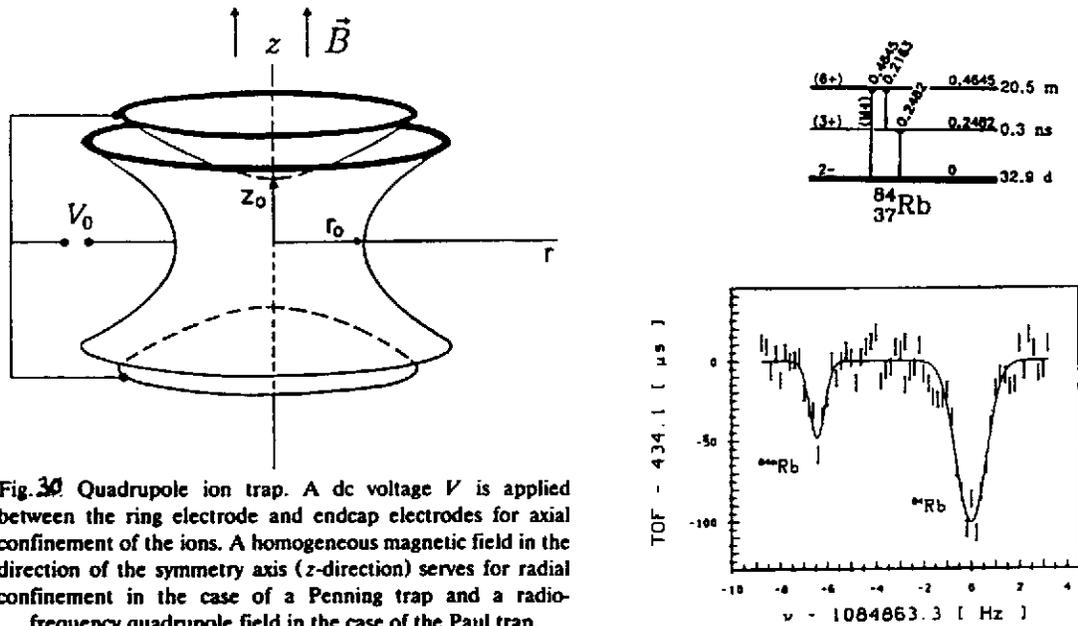
Fig. 30 Quadrupole ion trap. A dc voltage  $V$  is applied between the ring electrode and endcap electrodes for axial confinement of the ions. A homogeneous magnetic field in the direction of the symmetry axis (z-direction) serves for radial confinement in the case of a Penning trap and a radio-frequency quadrupole field in the case of the Paul trap.
