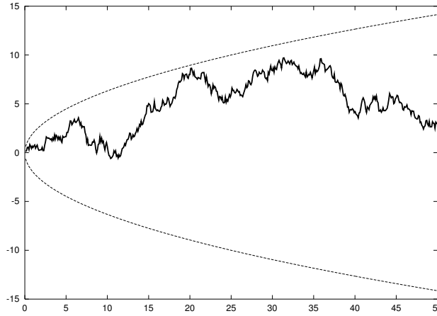
Figure 1.1: Simulation of a BM with the 95%-confidence interval curves f_{\pm}(t) = \pm 2\sqrt{t} .
