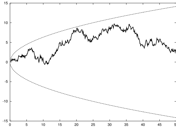
Figure 1.1: Simulation of a BM with the 95%-confidence interval curves f_{\pm}(t) = \pm 2\sqrt{t} .
