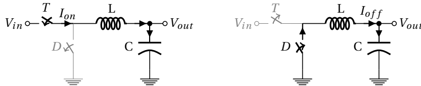
Figure 2.3: Simplified Buck converter circuit for the two configurations : left when the transistor T conducts (ON); right when it is OFF
