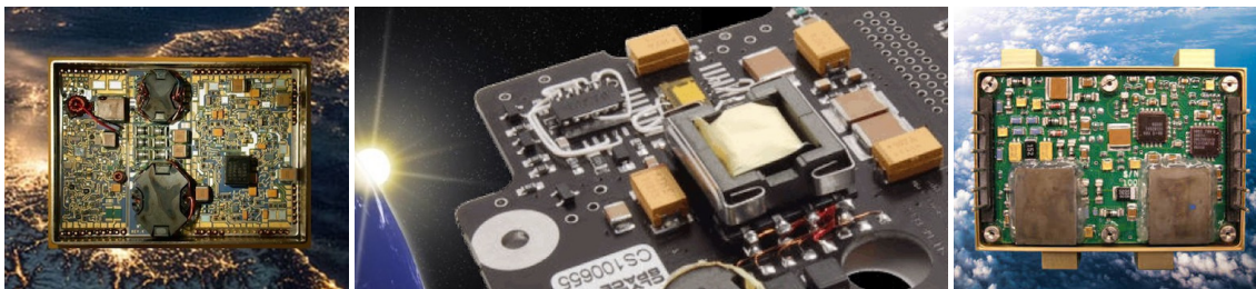
Figure 2.2: DC/DC converter for space application examples - APG & CLYDE SPACE & MICROCHIP
