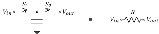
Figure 1.37: Equivalence between Resistor and Switched Capacitor.
