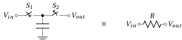
Figure 1.36: Equivalence between Resistor and Switched Capacitor.
