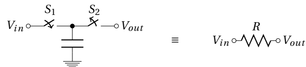
Figure 1.36: Equivalence between Resistor and Switched Capacitor.
