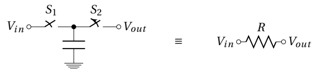
Figure 1.36: Equivalence between Resistor and Switched Capacitor.
