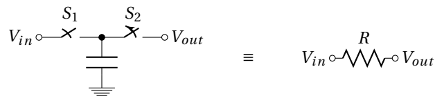
Figure 1.36: Equivalence between Resistor and Switched Capacitor.
