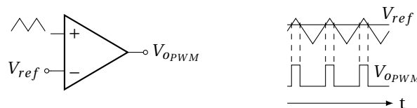
Figure 2.14: Simplified circuit of a Pulse Width Modulation (PWM).
