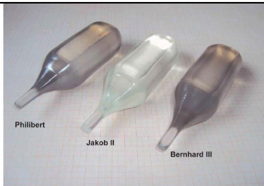
Fig. 5 Three CaWO 4 crystals from subsequent growth experiments weighing 853 g each, demonstrating the high reproducibility of the crystal growth procedure. The crystals at the left and the right are as-grown, while the clear crystal in the middle has already undergone an oxygenation treatment at 1450 °C in pure oxygen atmosphere followed by slow cooling. Note, the near square cross section of the crystals in their cylindrical part, as a result of the growth anisotropy.
