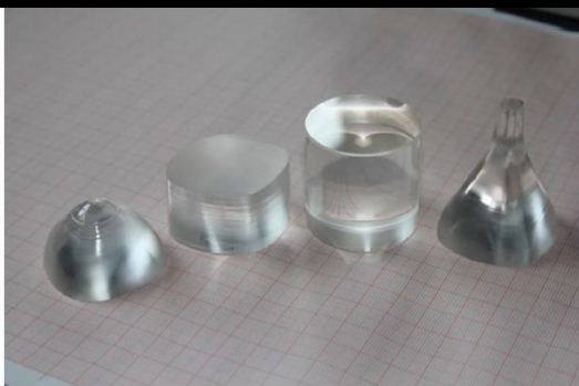
Fig. 4 Cut and polished pieces of the CaWO 4 crystal; from left to right: tail, residual cylinder, detector crystal, shoulder and neck.
