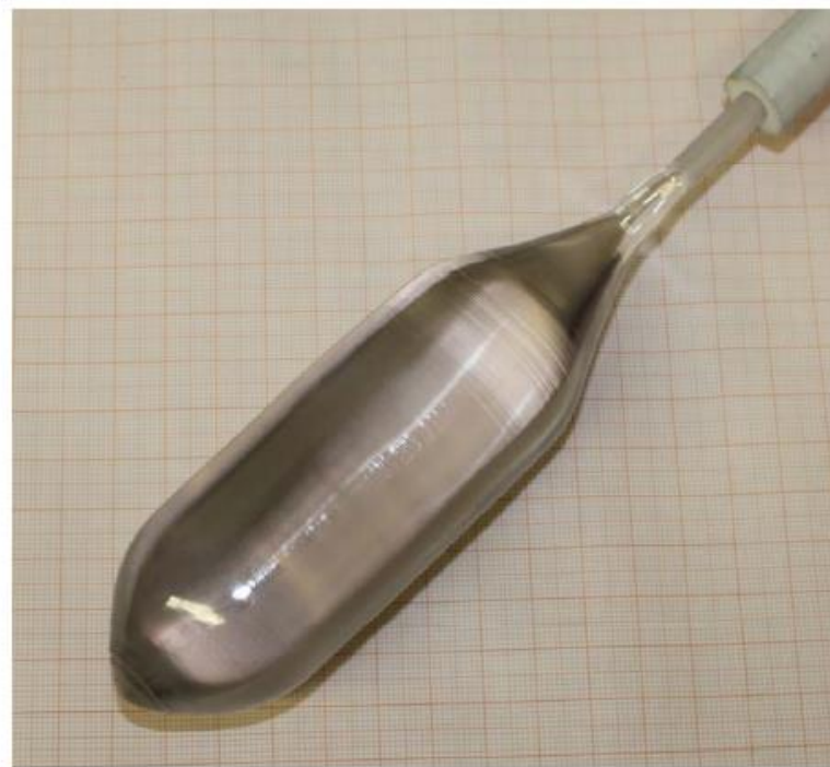
Fig. 2 CaWO 4 crystal of 886 g with seed holder and seed after growth. The slightly grey colour of the crystal is due to an oxygen deficiency originating from the low oxygen partial pressure in the growth atmosphere. The grey colour can be removed by a subsequent annealing procedure in pure oxygen at elevated temperatures.
