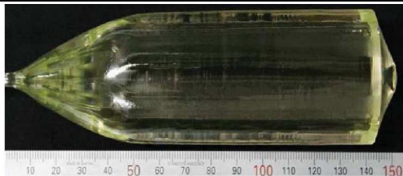
Fig. 18. 2 inch size \{\text{Tb}_3\}[\text{Sc}_{2-x}\text{Lu}_x](\text{Al}_3)\text{O}_{12} single crystal grown by the Czochralski technique, presented by Fujikura Ltd.
