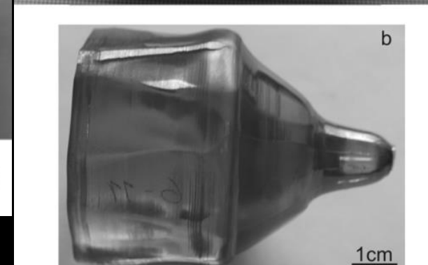
Fig. 2. BGO crystals grown by: a — LTG Cz technique, b — Cz technique.
