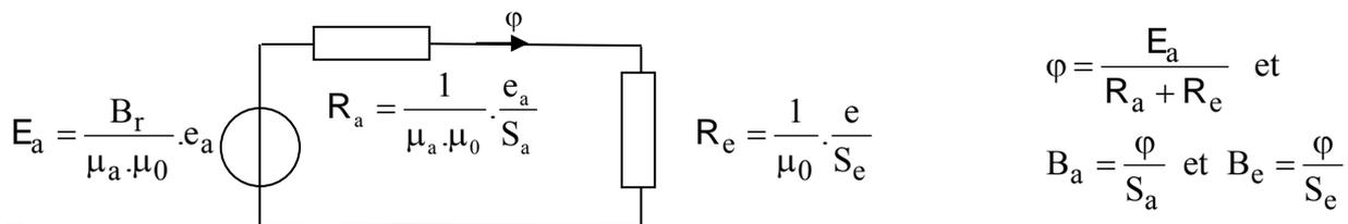
$$\phi = \frac{E_a}{R_a + R_e} \text{ et}$$
