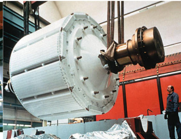
Rotor of the new, 100-MW (135,000-HP) synchronous motor
