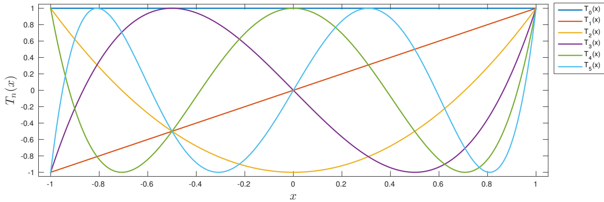
Figure 5. The first five Tchebyshev polynomials. Notice that T_n(-1) = (-1)^n and T_n(1) \equiv 1 .
