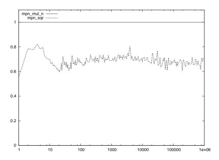
Figure 1.2 Ratio of the squaring and multiplication time for the GNU MP library, version 5.0.0, on a Core 2 processor, up to one million words.
