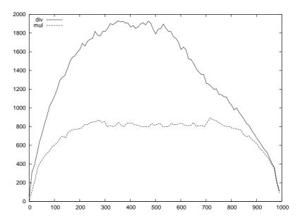
Figure 1.4 Time in  $10^{-5}$  seconds for the multiplication (lower curve) of x words by 1000-x words and for the division (upper curve) of 1000 words by x words, with GMP 5.0.0 on a Core 2 running at 2.83GHz.
