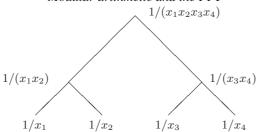
Figure 2.1 A recursive variant of Algorithm **MultipleInversion**. First go up the tree, building  $x_1x_2 \bmod N$  from  $x_1$  and  $x_2$  in the left branch,  $x_3x_4 \bmod N$  in the right branch, and  $x_1x_2x_3x_4 \bmod N$  at the root of the tree. Then invert the root of the tree. Finally, go down the tree, multiplying  $1/(x_1x_2x_3x_4)$  by the stored value  $x_3x_4$  to get  $1/(x_1x_2)$ , and so on.
