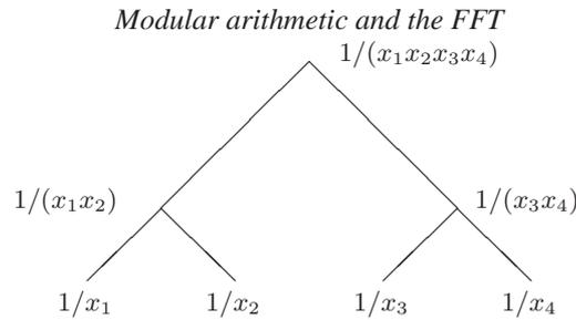
Figure 2.1 A recursive variant of Algorithm **MultipleInversion**. First go up the tree, building  $x_1x_2 \bmod N$  from  $x_1$  and  $x_2$  in the left branch,  $x_3x_4 \bmod N$  in the right branch, and  $x_1x_2x_3x_4 \bmod N$  at the root of the tree. Then invert the root of the tree. Finally, go down the tree, multiplying  $1/(x_1x_2x_3x_4)$  by the stored value  $x_3x_4$  to get  $1/(x_1x_2)$ , and so on.
