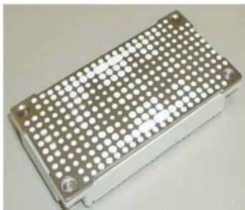
Fig. 6: Print image after blade squeezing
