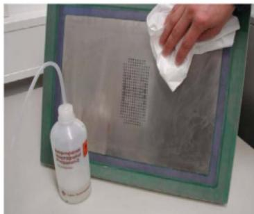
Fig. 3: Cleaning of the screen print template
