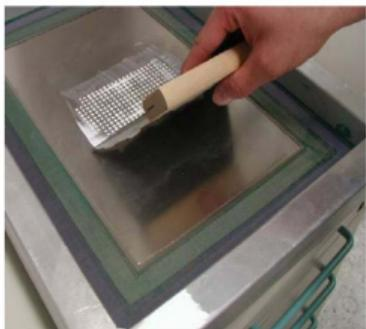
Fig. 5: Blade squeezing
