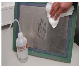
Fig. 3: Cleaning of the screen print template
