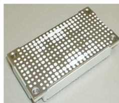
Fig. 6: Print image after blade squeezing
