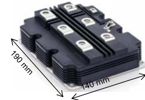
Ex. (Mitsubishi CM100HG-130XA) IGBT 6,5kV – 1000 A (24 kVA/cm 2 )
