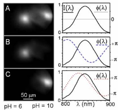
**Fig. 2 :** Experimental demonstration of pH-sensitive selective two-photon microscopy. The sample being imaged has an acidic (left side of the frame at pH 6) and a basic (right side of the frame at pH 10) region, both labeled with HPTS. The left panel shows the images obtained using 21-fs transform limited pulses centered at 842 nm (a) and shaped pulses with a spectral phase that maximize pH 6 (b) or pH 10 (c) fluorescence.
