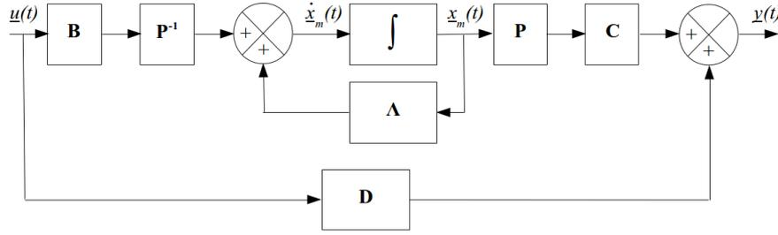
Figure 3.1: Modal decomposition of a transfer function
