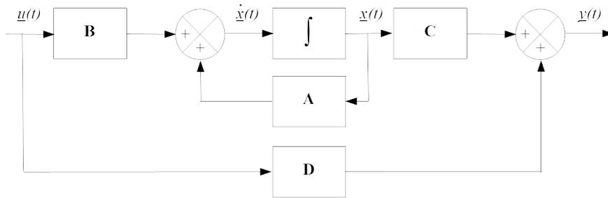
Figure 1.1: Block diagram of a state-space representation
