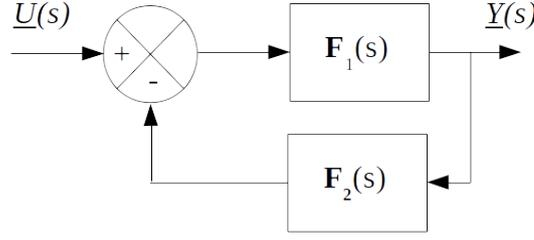
Figure 1.4: Feedback interconnection of systems
