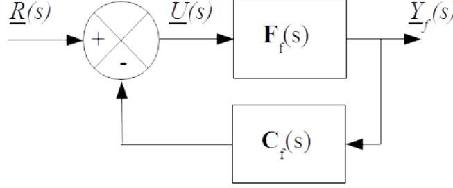
Figure C.3: Output feedback of the *fast* subsystem
