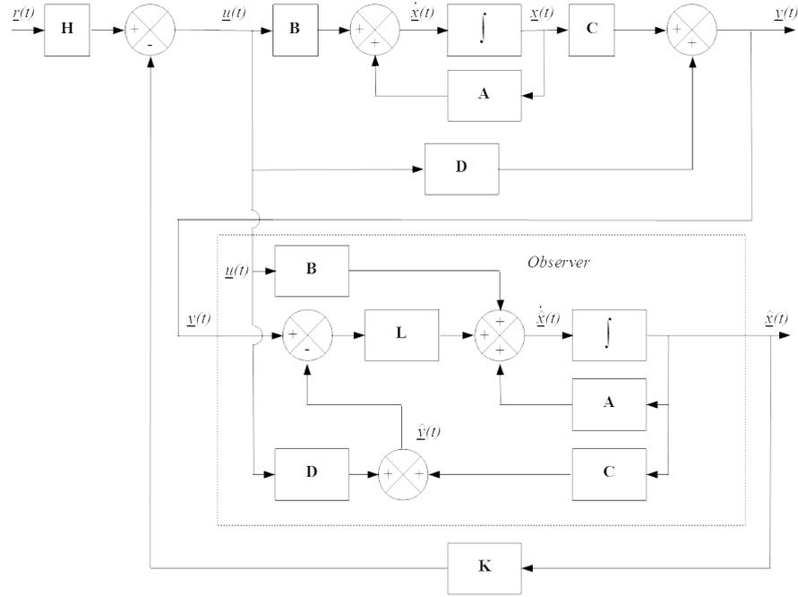
Figure 5.1: Block diagram of the observer-based controller
