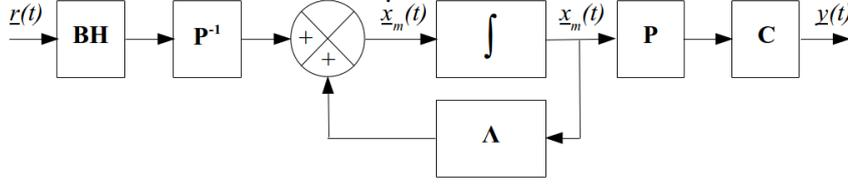
Figure 5.4: Modal decomposition of a transfer function
