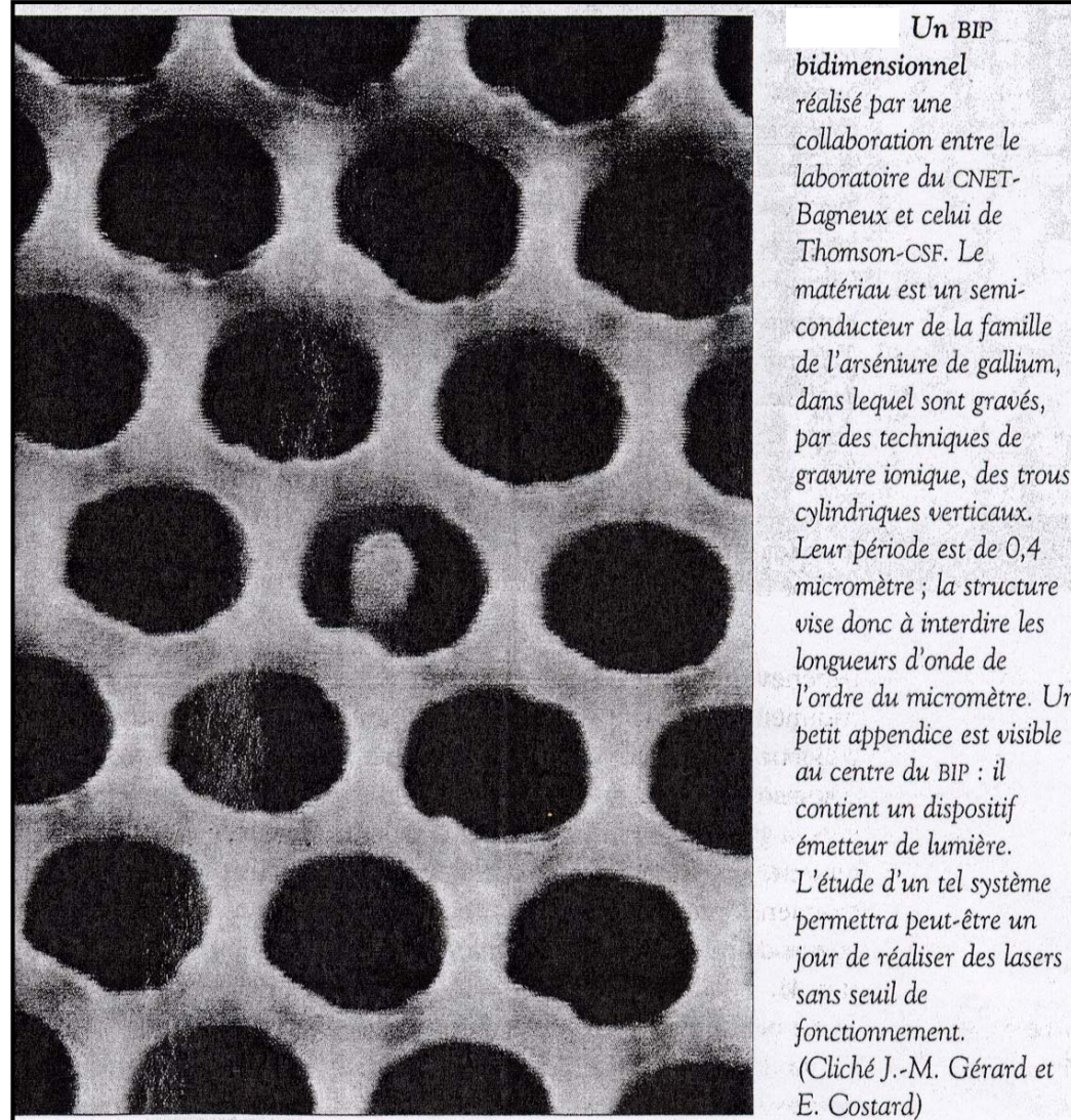
Hexagonal (or trigonal) 2D PBG-structures on GaAlAs (0.4 \mu m of lattice parameter)
