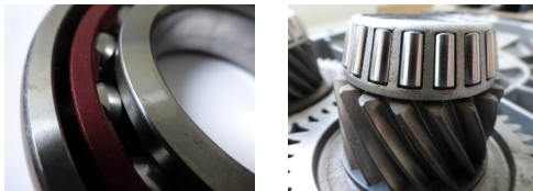
Figure: Examples of localized contacts: a) Ball bearing, b) Roller bearing and gear (Institut Pprime).
