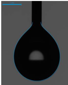
Figure: The pendant drop methods with contour identification
