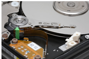
Figure: Example of surface adapted to phase shifting interferometry: hard drive disk surface
