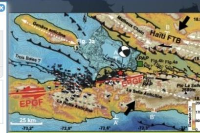
The authors of this new study, published in December 2015, used aerial images, high-resolution topographic data as well as bathymetry and geology data to identify the active faults in the epicentral zone. They also demonstrated the existence of a new structure, the Lamentin thrust. This is a thrust of south-eastern/north-western azimuth, dipping southward, north of the EPGF, in Port-au-Prince bay. It is
