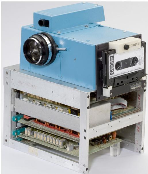
**Fig. I.1.** The very first digital camera created by Steven Sasson in 1973. This prototype was the basis for the US patent issued on December 26th, 1978. <https://lens.blogs.nytimes.com/2015/08/12/kodaks-first-digital-moment/>
