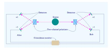
Scheme of a "two-channel" Bell test The source S produces pairs of photons, sent in opposite directions. Each photon encounters a two-channel polariser whose orientation (a or b) can be set by the experimenter. Emerging signals from each channel are detected and coincidences counted by the coincidence monitor. https://en.wikipedia.org/wiki/Bell's\_theorem.
