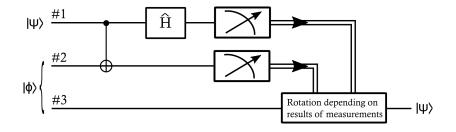
*Remark:* if qubit #1 is measured in state  $|1\rangle$ , one should apply  $\hat{Z}$ , nothing otherwise. If qubit #2 is measured in state  $|1\rangle$ , one should apply  $\hat{X}$ , nothing otherwise.
